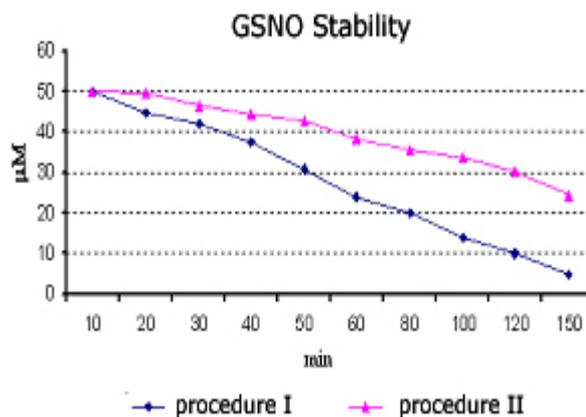
Graph 1. The stability of GSNO synthesized according to procedure I (in aqueous solution) and procedure II (sedimentation). The reduction of GSNO concentration was monitored in a phosphate buffer (pH-7.4) by spectrophotometric absorbance determination at  $\lambda_{\text{max}}=334\text{nm}$ .
