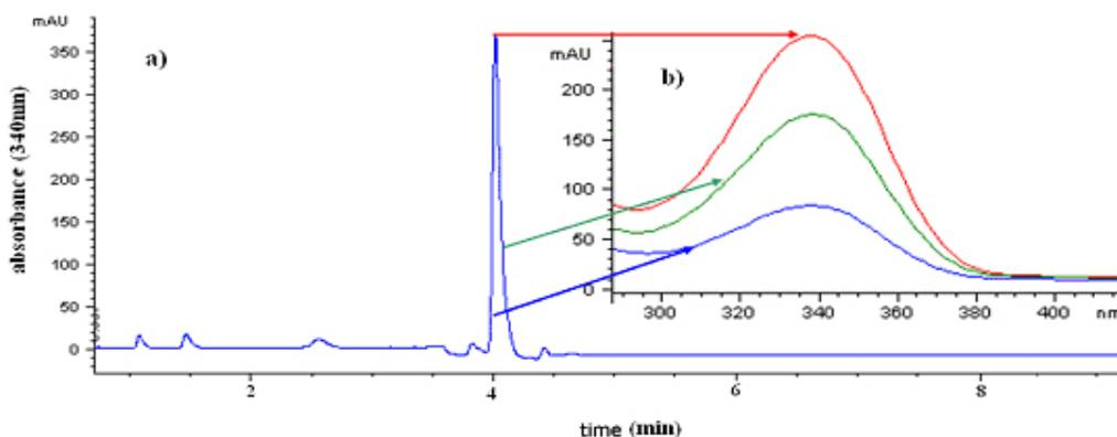
Figure 1. a) HPLC chromatogram of GSNO solution synthesized according to procedure II b) absorption spectrum of S-nitrosogluthione peak
