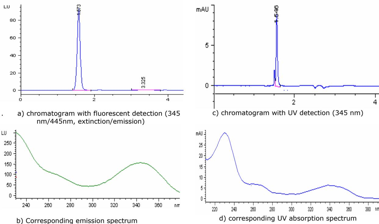
Figure 3. HPLC chromatograms of GSNO-OPA-ME. 500  $\mu\text{L}$  GSNO (50  $\mu\text{M}$ ) + 100  $\mu\text{L}$  OPA reagent B (OPA + ME), injected 20  $\mu\text{L}$
