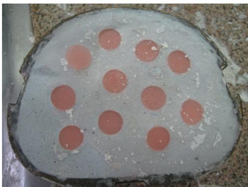
Figure 1. Polymerization of the heat polymerized acrylic samples in standard metal flask (Changsha Zhongbang Medical Instruments Co., China).
