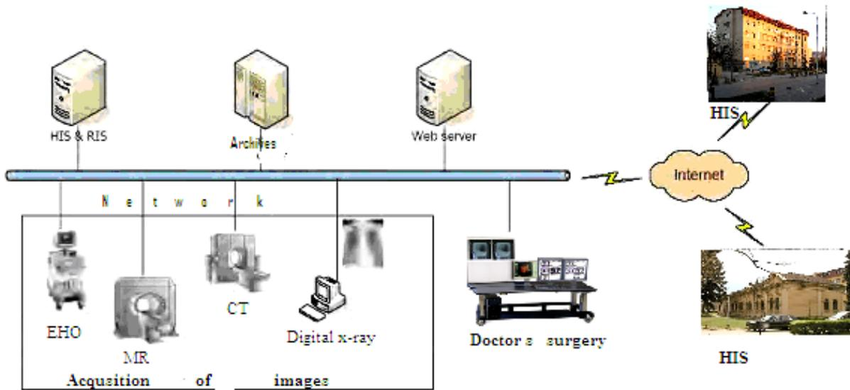
Figure 3. Picture Archiving and Communication System (PACS) components
