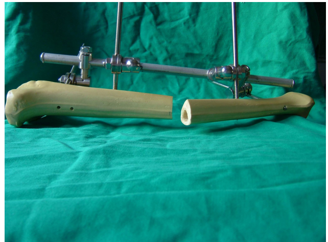
Figure 5. Corrections of varus and valgus by external skeletal fixator on a bone model
