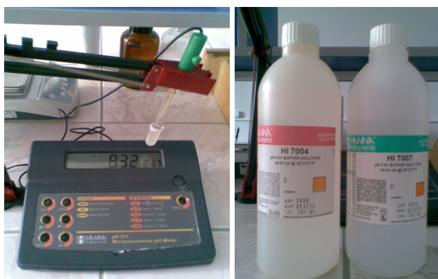
Figure 2. Microprocessor pH Meter HANNA instruments and standard buffer solutions for pH meter calibration ( \text{pH}=4.1 i \text{pH}=7.1 )
