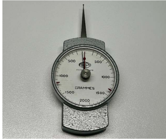
Figure 3. Digital dynamometer used for precise measurement of retention force (grams (g) converted to Newtons (N)).
