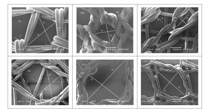
Figure 1. Scan electron microscope graft images (50/1) (I-HWPP, II-LWPP, III-MPP, IV-MPPG, V-CPP, VI-TPP, Š-pore size, D-pore length, DV-filament thickness)
