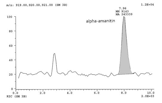
Figure 2. Typical chromatogram of alpha-amanitin standard, 25 ng/mL, Single Ion Monitoring mod (SIM)
