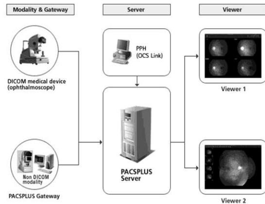
**Figure 1.** Ophthalmic PACS configuration
