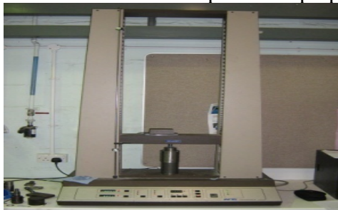
Slika 3. Univerzalni stroj za testiranje "Instron" (model 1193, Instron corp., USA) Figure 3. Universal Testing Machine (Instron Universal Testing Machine model 1193, Instron Corp., Canton, USA)
